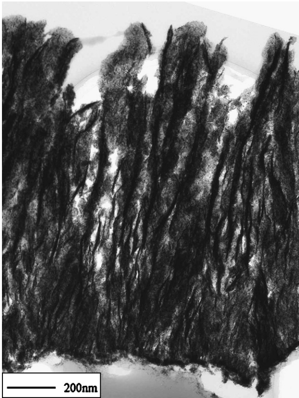
Fig. 3. TEM photographs of the dendritic Pt film at the magnitude of \times 100,000 .
